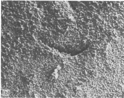
Figure 5 Large cracks in the presence of PbO in PZT specimens.
